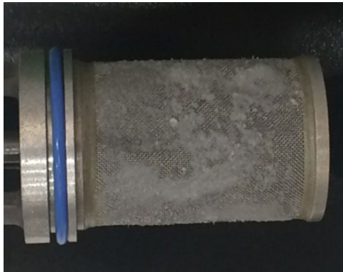
Figure 3. Aircraft Fuel Filters with DEF Contamination
