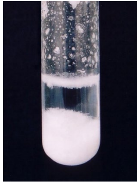
Figure 2. DEF Crystalline Deposits Formed when Mixed with Jet Fuel
