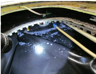
Figure 4. DEF Deposits in Aircraft Fuel Tank
